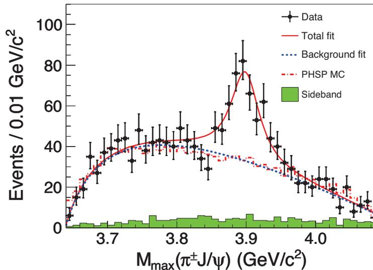
**Figure 78.4:** The  $\pi^\pm J/\psi(1S)$  invariant mass distribution from BESIII [78]  $e^+e^-$  collision data taken at a center-of-mass energy near 4260 MeV.
