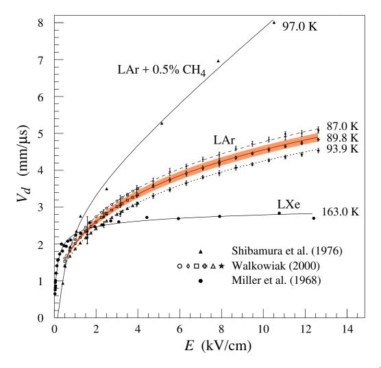
Figure 35.25: Drift velocity of free electrons as a function of electric field strength for LAr [260], LAr + 0.5% CH<sub>4</sub> [261] and LXe [262]. The average temperatures of the liquids are indicated. Results of a fit to an empirical function [263] are superimposed. In case of LAr at 91 K the error band for the global fit [260] including statistical and systematic errors as well as correlations of the data points is given. Only statistical errors are shown for the individual LAr data points.
