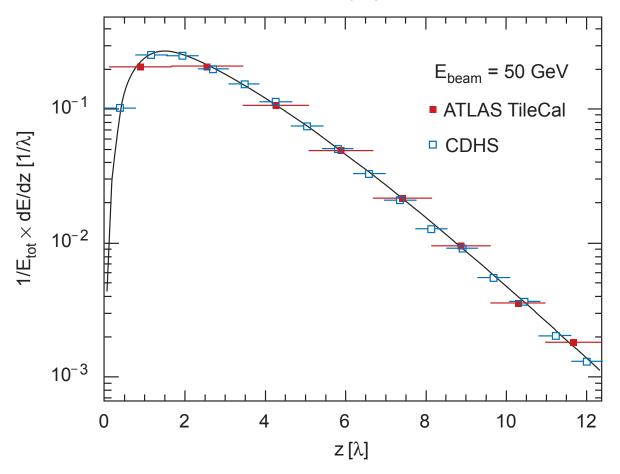
Figure 35.24: Mean profiles of  $\pi^+$  (mostly) induced cascades in the CDHS neutrino detector [255] and in the ATLAS tile calorimeter [224]. Measurements are front of the calorimeter, and so are convoluted with the first interaction distance.
