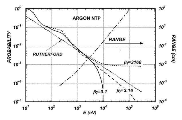
Figure 35.3: Probability of single collisions in which released electrons have an energy E or larger (left scale) and practical range of electrons in Ar/CH<sub>4</sub> (P10) at NTP (dot-dashed curve, right scale) [88].
