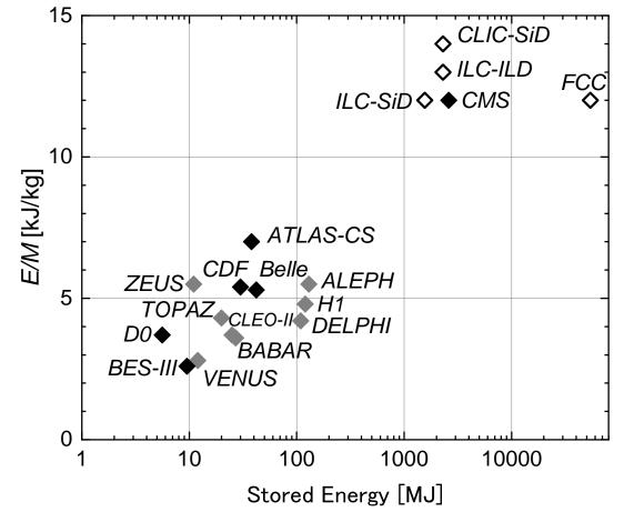
Figure 35.27: Ratio of stored energy to cold mass for major detector solenoids. Gray indicates magnets no longer in operation.
