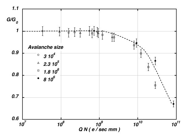
Figure 35.8: Charge rate dependence of normalized gas gain  $G/G_0$  (relative to zero counting rate) in proportional thin-wire detectors [111]. Q is the total charge in single avalanche; N is the particle rate per wire length.
