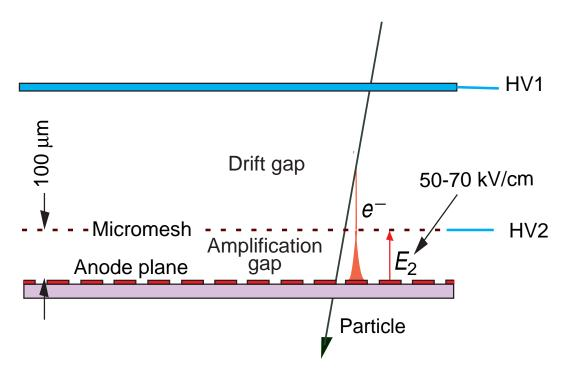
Figure 35.11: Schematic drawing of the Micromegas detector.
