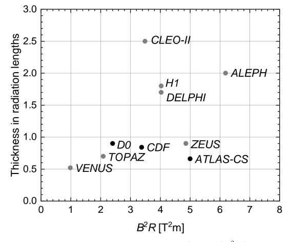
Figure 35.26: Magnet wall thickness in radiation length as a function of  $B^2R$  for various detector solenoids. Gray entries are for magnets no longer in use, and entries underlined are not listed in Table 35.11. Open circles are for magnets not designed to be "thin." The SSC-SDC prototype provided important R&D for LHC magnets.
