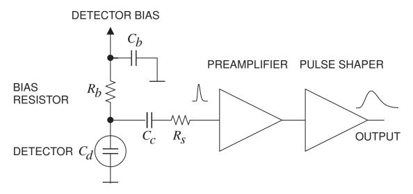
Figure 35.18: Typical detector front-end circuit.
