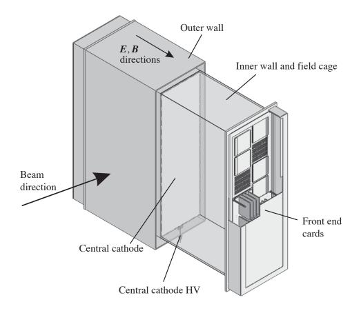
Figure 35.14: One of the 3 TPC modules for the near detector of the T2K experiment [134]. The size is  $2 \times 2 \times 0.8 \text{ m}^3$ . Micromegas devices are used for gas amplification and readout.
