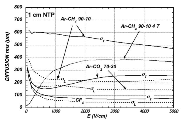
Figure 35.5: Electron longitudinal diffusion  $(\sigma_L)$  (dashed lines) and transverse diffusion  $(\sigma_T)$  (full lines) for 1 cm of drift at NTP and B = 0. The dotted line shows  $\sigma_T$  for the P10 mixture at 4 T [87].
