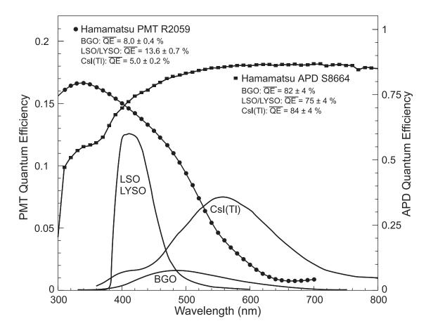
Figure 35.2: The quantum efficiencies of two photodetectors, a Hamamatsu R2059 PMT with bialkali cathode and a Hamamatsu S8664 avalanche photodiode (APD), are shown as a function of wavelength. Also shown in the figure are emission spectra of three crystal scintillators, BGO, LSO and CsI(Tl), and the numerical values of the emission weighted quantum efficiencies. The area under each emission spectrum is proportional to crystal's light yield.
