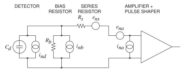
Figure 35.19: Equivalent circuit for noise analysis.
