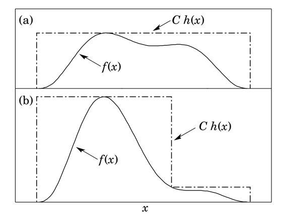
Figure 41.2: Illustration of the acceptance-rejection method. Random points are chosen inside the upper bounding figure, and rejected if the ordinate exceeds f(x). The lower figure illustrates a method to increase the efficiency (see text).
