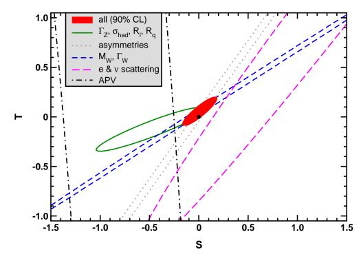
Figure 10.6: 1  $\sigma$  constraints (39.35%) on S and T (for U = 0) from various inputs combined with  $M_Z$ . S and T represent the contributions of new physics only. Data sets not involving  $M_W$  or  $\Gamma_W$  are insensitive to U. With the exception of the fit to all data, we fix  $\alpha_s = 0.1185$ . The black dot indicates the Standard Model values S = T = 0.
