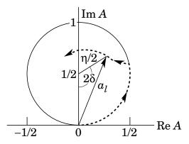
Figure 46.7: Argand plot showing a partial-wave amplitude  $a_{\ell}$  as a function of energy. The amplitude leaves the unitary circle where inelasticity sets in  $(\eta_{\ell} < 1)$ .
