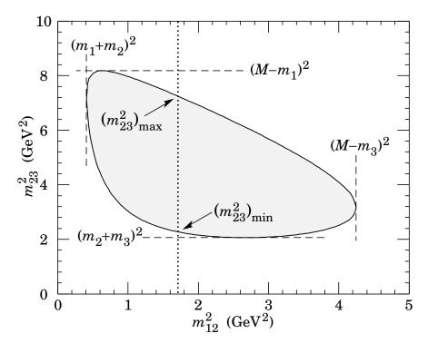
**Figure 46.3:** Dalitz plot for a three-body final state. In this example, the state is  $\pi^+\overline{K}{}^0p$  at 3 GeV. Four-momentum conservation restricts events to the shaded region.
