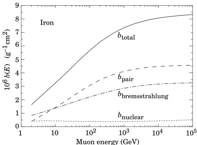
**Figure 32.22:** Contributions to the fractional energy loss by muons in iron due to  $e^+e^-$  pair production, bremsstrahlung, and photonuclear interactions, as obtained from Groom *et al.* [5] except for post-Born corrections to the cross section for direct pair production from atomic electrons.
