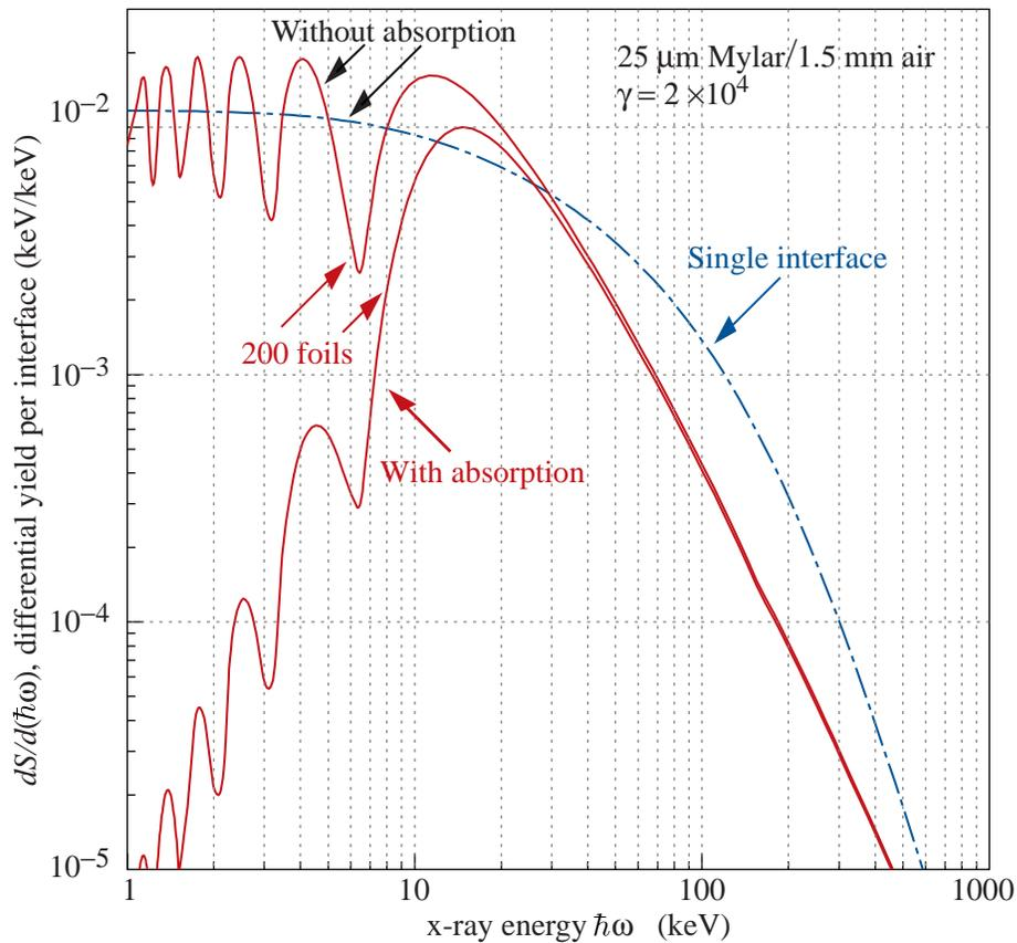
**Figure 32.27:** X-ray photon energy spectra for a radiator consisting of 200 25  $\mu\text{m}$  thick foils of Mylar with 1.5 mm spacing in air (solid lines) and for a single surface (dashed line). Curves are shown with and without absorption. Adapted from Ref. 88.
