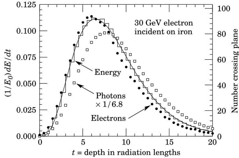
**Figure 32.20:** An EGS4 simulation of a 30 GeV electron-induced cascade in iron. The histogram shows fractional energy deposition per radiation length, and the curve is a gamma-function fit to the distribution. Circles indicate the number of electrons with total energy greater than 1.5 MeV crossing planes at  $X_0/2$  intervals (scale on right) and the squares the number of photons with  $E \geq 1.5$  MeV crossing the planes (scaled down to have same area as the electron distribution).
