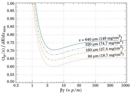
**Figure 32.9:** Most probable energy loss in silicon, scaled to the mean loss of a minimum ionizing particle, 388 eV/ $\mu$ m (1.66 MeV g<sup>-1</sup>cm<sup>2</sup>).
