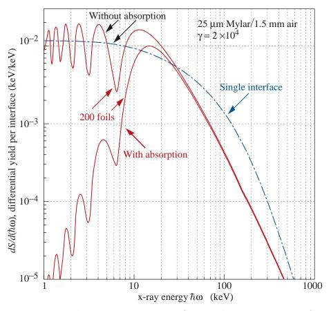
Figure 32.27: X-ray photon energy spectra for a radiator consisting of 200 25  $\mu$ m thick foils of Mylar with 1.5 mm spacing in air (solid lines) and for a single surface (dashed line). Curves are shown with and without absorption. Adapted from Ref. 88.
