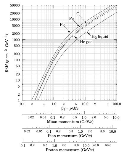
**Figure 32.4:** Range of heavy charged particles in liquid (bubble chamber) hydrogen, helium gas, carbon, iron, and lead. For example: For a  $K^+$  whose momentum is 700 MeV/c,  $\beta\gamma=1.42$ . For lead we read  $R/M\approx 396$ , and so the range is 195 g cm<sup>-2</sup> (17 cm).
