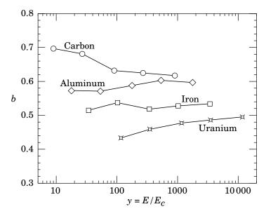
**Figure 32.21:** Fitted values of the scale factor b for energy deposition profiles obtained with EGS4 for a variety of elements for incident electrons with  $1 \le E_0 \le 100$  GeV. Values obtained for incident photons are essentially the same.
