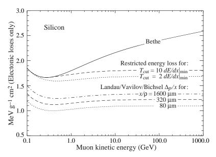
Figure 32.6: Bethe dE/dx, two examples of restricted energy loss, and the Landau most probable energy per unit thickness in silicon. The change of  $\Delta_p/x$  with thickness x illustrates its  $a \ln x + b$  dependence. Minimum ionization  $(dE/dx|_{\min})$ is  $1.664 \text{ MeV g}^{-1} \text{ cm}^2$ . Radiative losses are excluded. The incident particles are muons.
