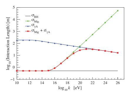
Figure 32.19: Interaction length for a photon in ice as a function of photon energy for the Bethe-Heitler (BH), LPM (Mig) and photonuclear ( $\gamma A$ ) cross sections [56]. The Bethe-Heitler interaction length is  $9X_0/7$ , and  $X_0$  is 0.393 m in ice.
