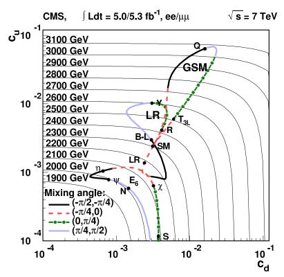
**Figure 2:** CMS results from [23]. Limits in the  $c_u^{\ell} - c_d^{\ell}$  plane ( $\ell = e$  or  $\mu$ ) are shown as thin lines for certain  $M_{Z'}$  values. For specific sets of charges (described in [6]), parametrized by a mixing angle, the mass limit is given by the intersection of the thick and thin lines.
