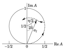
**Figure 45.7:** Argand plot showing a partial-wave amplitude  $a_{\ell}$  as a function of energy. The amplitude leaves the unitary circle where inelasticity sets in  $(\eta_{\ell} < 1)$ .
