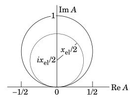
**Figure 45.8:** Argand plot for a resonance.
