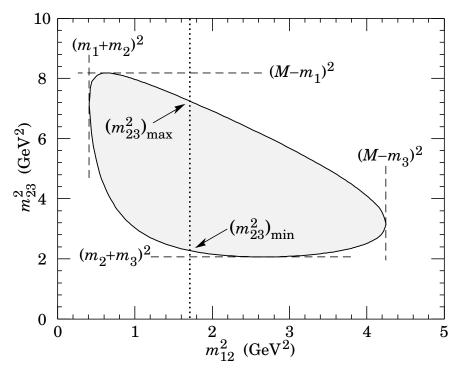
Figure 45.3: Dalitz plot for a three-body final state. In this example, the state is  $\pi^+ \overline{K}{}^0 p$  at 3 GeV. Four-momentum conservation restricts events to the shaded region.
