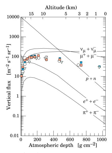
**Figure 26.3:** Vertical fluxes of cosmic rays in the atmosphere with E > 1 GeV estimated from the nucleon flux of Eq. (26.2). The points show measurements of negative muons with  $E_{\mu} > 1$  GeV [32–36].
