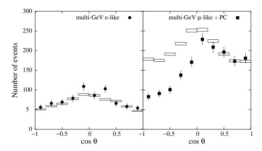
**Figure 26.7:** Zenith-angle dependence of multi-GeV neutrino interactions from SuperKamiokande [68]. The shaded boxes show the expectation in the absence of any oscillations.
