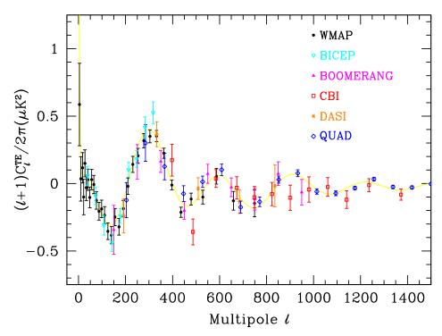
**Figure 23.3:** Cross power spectrum of the temperature anisotropies and Emode polarization signal from WMAP, together with estimates from BICEP, BOOMERANG, CBI, DASI, and QUAD, several of which extend to higher  $\ell$ . Note that the y-axis here is not multiplied by the additional  $\ell$ , which helps to show both the large and small angular scale features.
