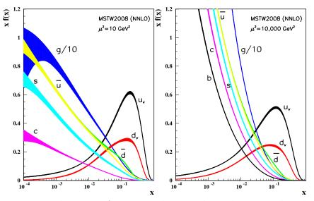
Figure 16.4: Distributions of x times the unpolarized parton distributions f(x)(where  $f = u_v, d_v, \overline{u}, \overline{d}, s, c, b, g$ ) and their associated uncertainties using the NNLO MSTW2008 parameterization [13] at a scale  $\mu^2 = 10 \text{ GeV}^2$  and  $\mu^2 = 10,000 \text{ GeV}^2$ .
