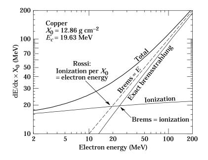
Figure 26.11: Two definitions of the critical energy  $E_c$ .
