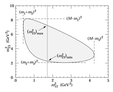
Figure 35.3: Dalitz plot for a three-body final state. In this example, the state is  $\pi^+ K^0 p$  at 3 GeV. Four-momentum conservation restricts events to the shaded region.
